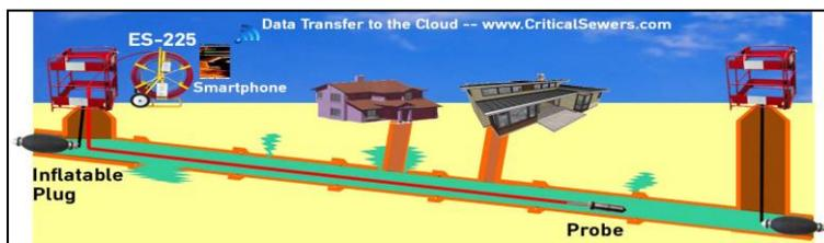
Electro Scan technology was able to inspect pipes that were suspected of being subject to ground water infiltration where previous CCTV inspections had failed to identify the source due to visual issues, obstructions &
